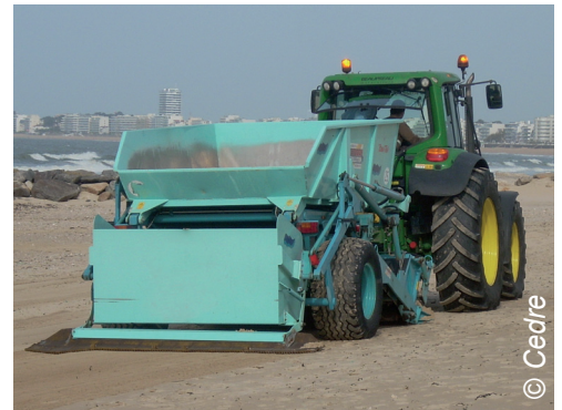
Large beach-cleaning machine powered by a tractor
